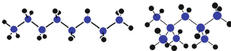
Fig. 1.8 Straight n-octane, left , has a higher tendency to autoignite than isooctane, right
