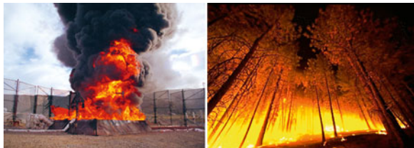
Fig. 7.9 A liquid pool fire (Sandia National Laboratories) and forest fire (USDA Forest Service) serve as examples of condensed-fuel non-premixed flames
